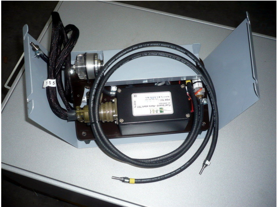
engine fuel board with pump, valves, filter and flow meter
