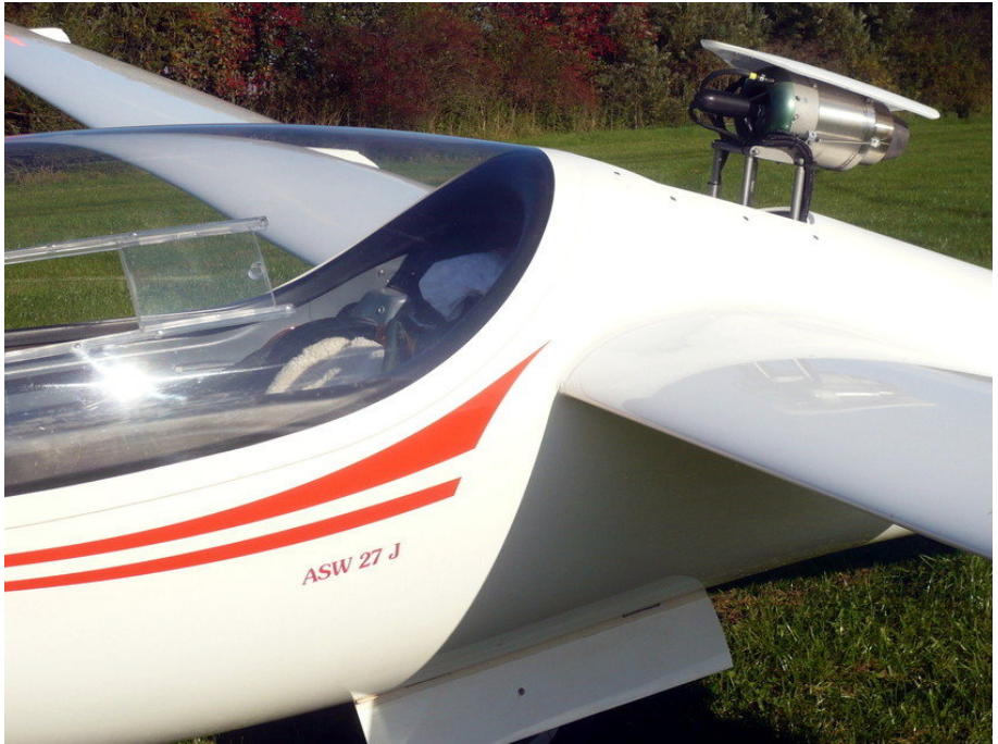
ASW27-J after 45 engine starts and 3,3 hours engine runtime
