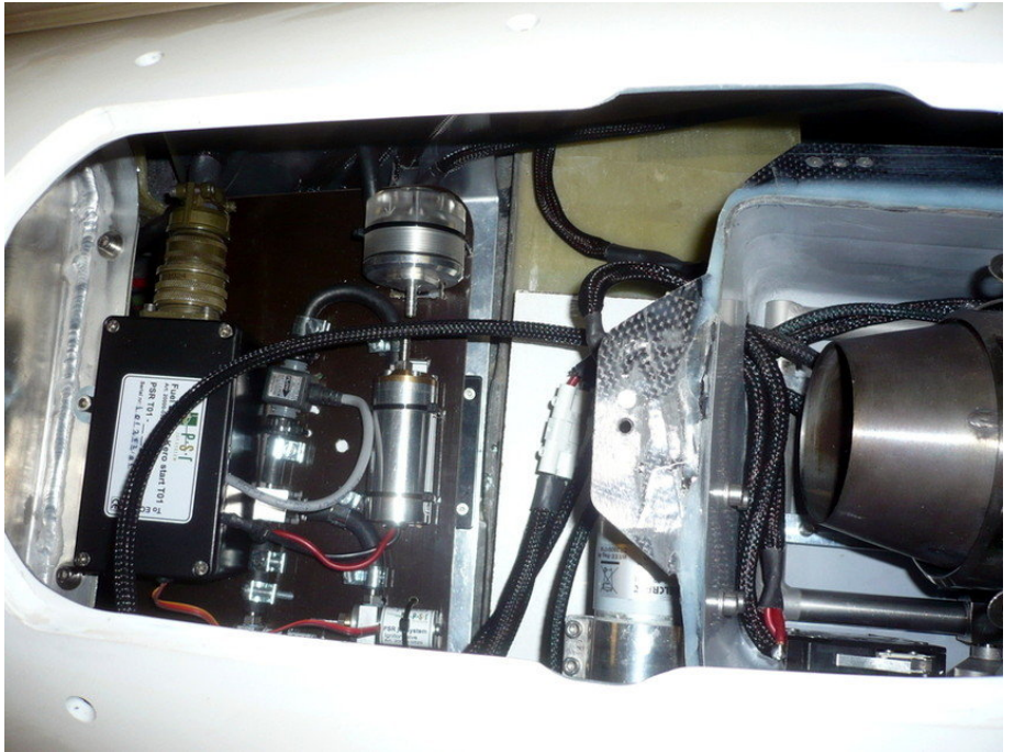
engine and engine fuel board during installation
