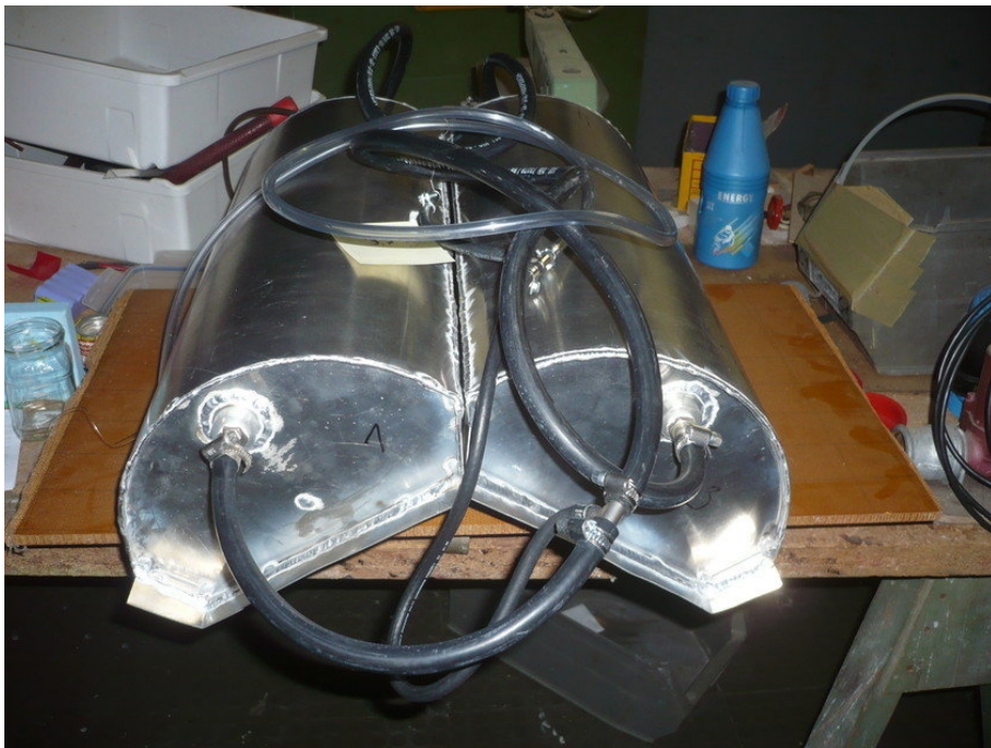
two 4 gallons aluminium tanks
