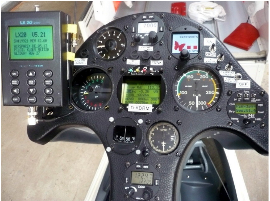
instrument panel with engine service data terminal
